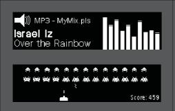
The display of the aquaero can be used for external data like media player information. You can display information with up to 20 fps. These screens with external data can be shown alternately to the screens of the aquaero. At the moment we are developing a driver for the popular LCD-Hype software. While displaying animations the aquaero still works in the background and all menus can be used.
