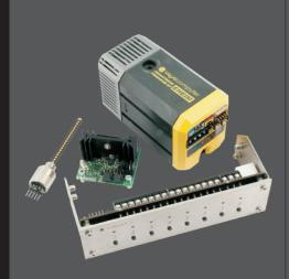
poweradjust 2: the poweradjust 2 device was developed simultaneously to the new aquaero and fits to it perfectly. By connecting the poweradjust 2 to the aquaero it will have another powerful amplifier incl. voltage regulation and temperature measuring. There will be another temperature sensor and a flow meter integrated to the aquaero sensor structure.
