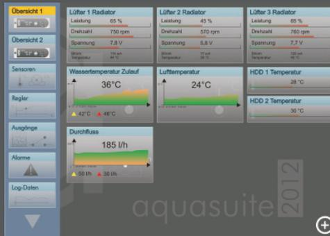
The aquasuite software has been redesigned. Now it has a complete new graphical interface for device management. You can analyze all data in real time or transfer the internal aquaero cache into the aquasuite database.
