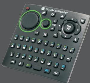
The so called aquaremote, a IR remote with a small keyboard, a mouse-pad and multimedia keys, gives you the opportunity to control your PC. The current key level (shift, control, etc.) will be displayed in the aquaero through a pop-up window. The mouse can be controlled by a pad with 8 integrated buttons. Mouse strikes with pressed mouse buttons are possible and the keyboard is also usable in the BIOS Setup.
