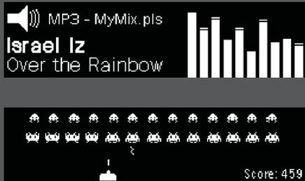
The display of the aquaero can be used for external data like media player information. You can display information with up to 20 fps. These screens with external data can be shown alternately to the screens of the aquaero. At the moment we are developing a driver for the popular LCD-Hype software. While displaying animations the aquaero still works in the background and all menus can be used.
