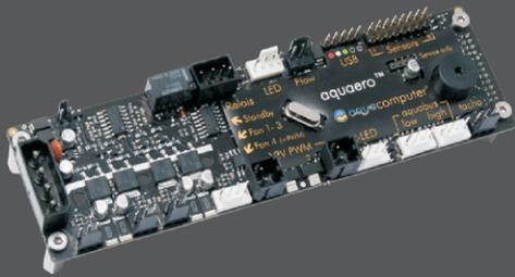
Besides all the other functions of the aquaero it has 2 aquabus interfaces. Through the aquabus connection you will be able to link other Aqua Computer devices to the aquaero. All the other linked devices will be identified and integrated as a part of the aquaero. There are no separate device menus in the aquaero anymore.
