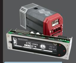
The aquastream ULTIMATE features an integrated water temperature sensor. In addition, an external temperature sensor can be connected to the pump. If an Aqua Computer flow sensor is connected to the unit, it is possible to monitor the flow rate of the system.
